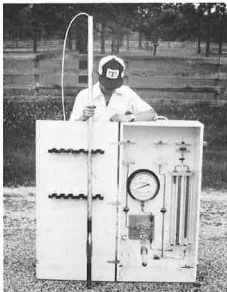
Figure 3. Components of pavement pressuremeter.
