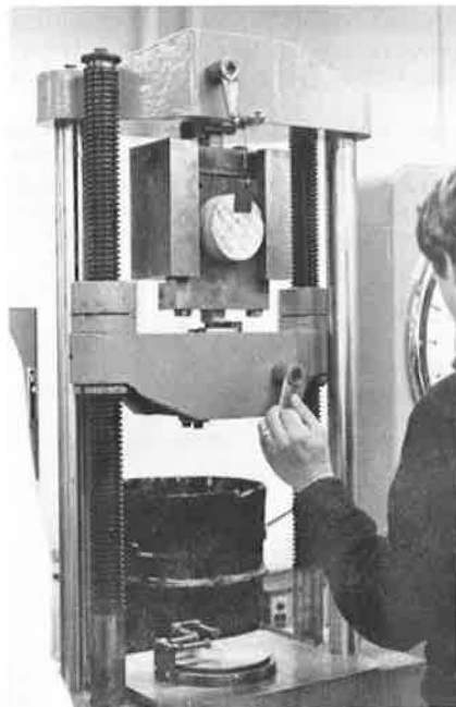
Figure 2. Hydraulic testing machine, jig, and specimen.
