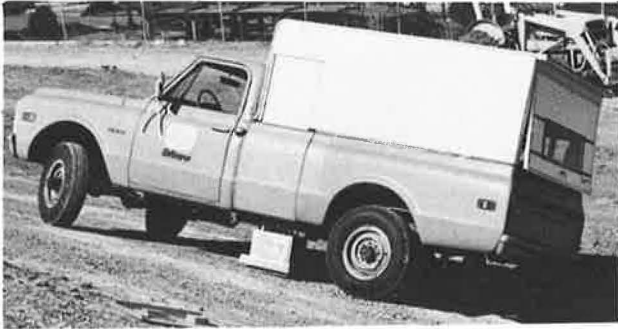
Figure 7. Testing on inclined embankment with probe in full inboard position.
