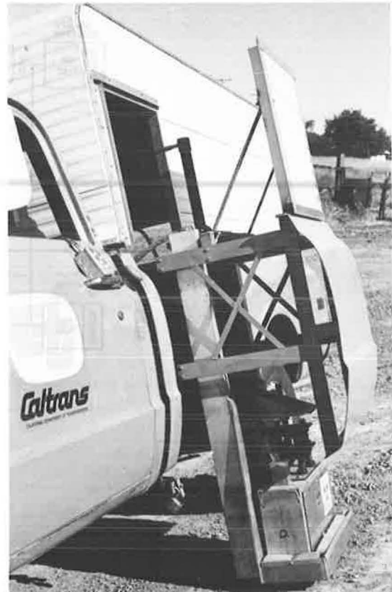
Figure 5. Testing of probe positioning with mechanism fully extended.
