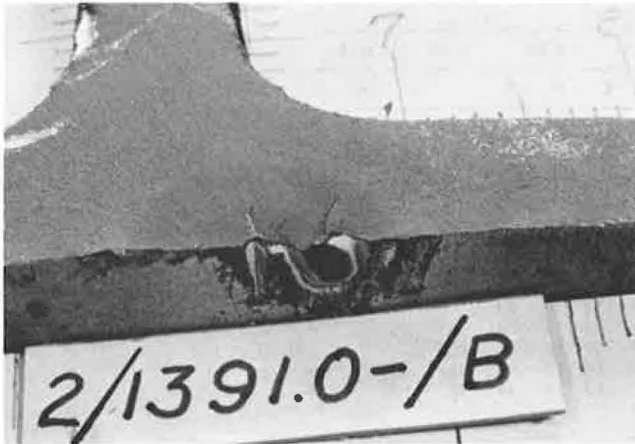
Figure 8. Fatigue crack initiated by heat stamp.
