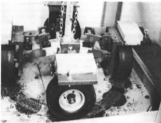
Figure 6. North Carolina small-wheel circular-track wear and polish machine.
