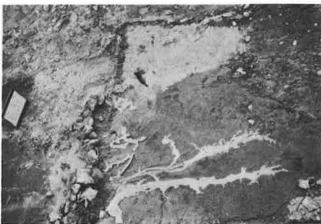
Figure 22. Channeling marks at interface between concrete slab and cement-treated base.
