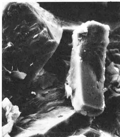
Figure 7. SEM photograph (1000x) of aggregate 2 (Niemann, Lamont, Iowa).
