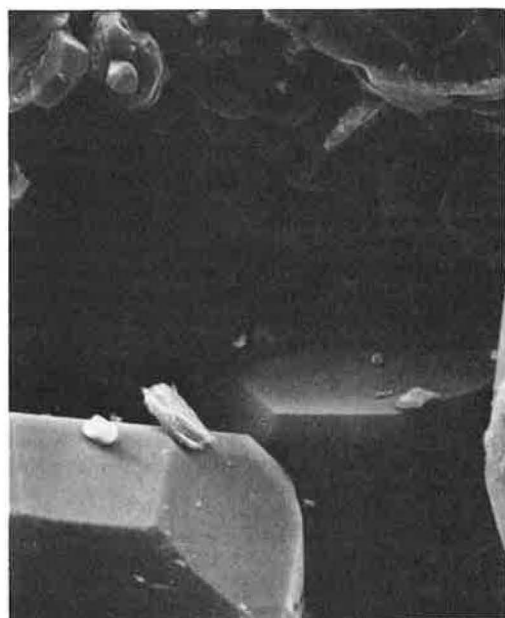
Figure 6. SEM photograph (1000x) of aggregate 1 (Weaver, Alden, Iowa).
