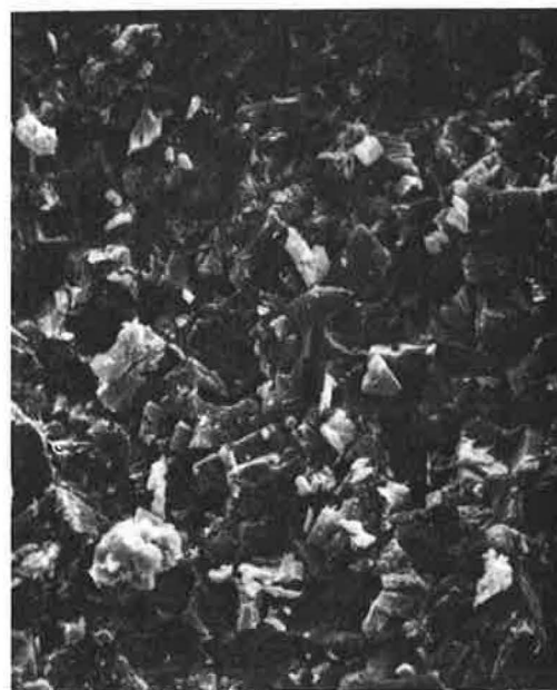
Figure 9. SEM photograph (1000x) of aggregate 10 [Alpha, Prairieburg, Iowa (Plower)].
