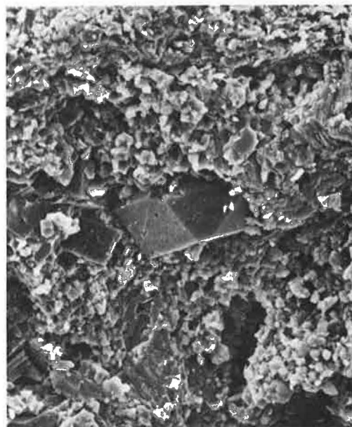
Figure 8. SEM photograph (1000x) of aggregate 9 (Columbia, Ullin, Illinois).
