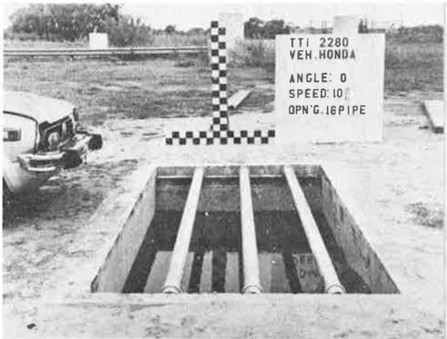
Figure 4. Test pit with 16-in grate spacing.
