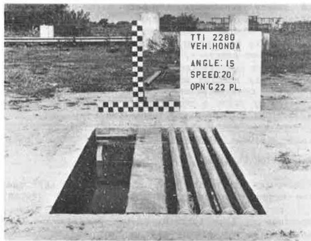
Figure 2. Test pit installation.
