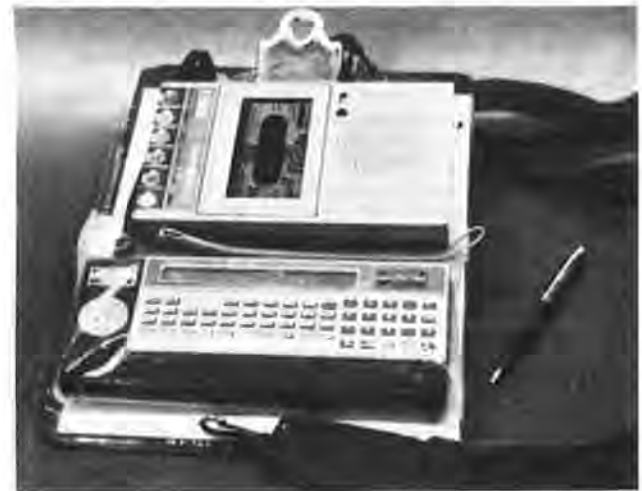
Figure 2. Computerized data collection field package which interfaces to microcomputer system.
