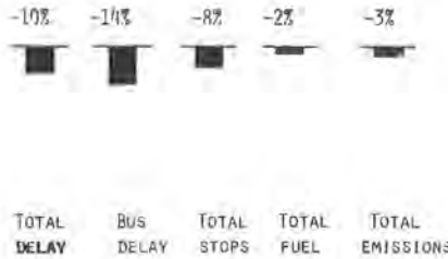
Figure 5. Effect of optimized splits and offsets on reducing impact under existing flow conditions.
