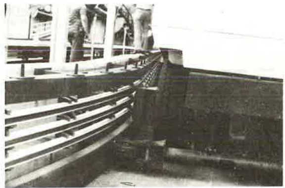
Figure 4. Power collector, pneumatic tire, and lateral wheels.
