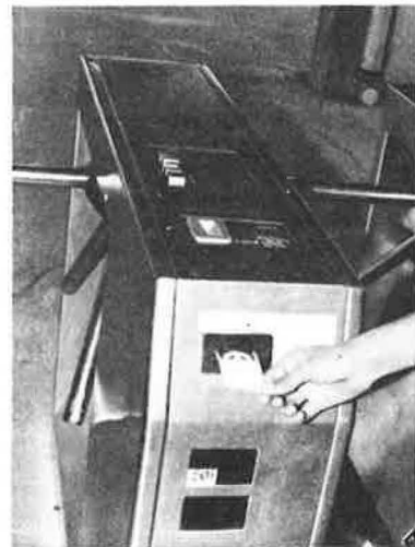
Figure 8. Automated fare gate.
