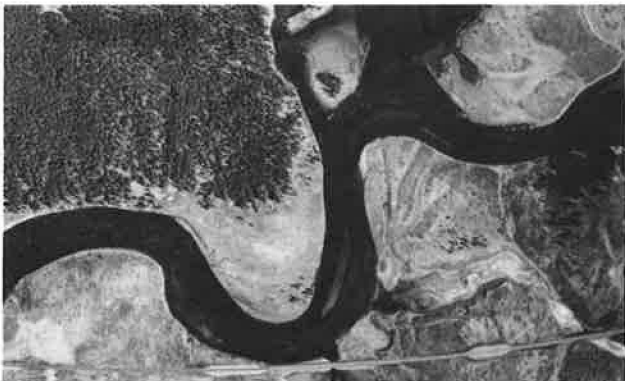
Figure 6. Aggradation on Yellowstone River in Yellowstone National Park, illustrated by deposition at confluences and culverts.
