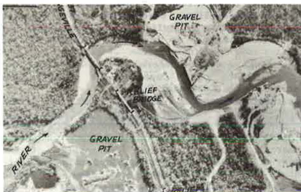
Figure 3. Degradation due to gravel mining upstream and downstream on Amite River at LA-37 near Grangeville, Louisiana.
