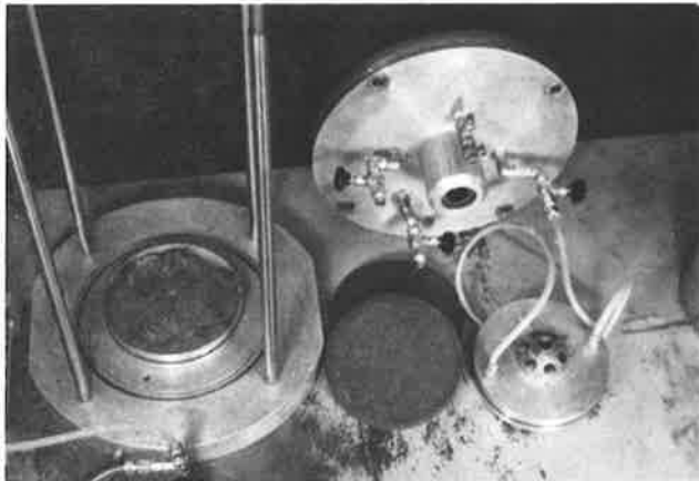
Figure 2. Triaxial cell parts. [Shown (from left to right) are the cell base, loading cap, and porous stone; the cell cap is in the back.]
