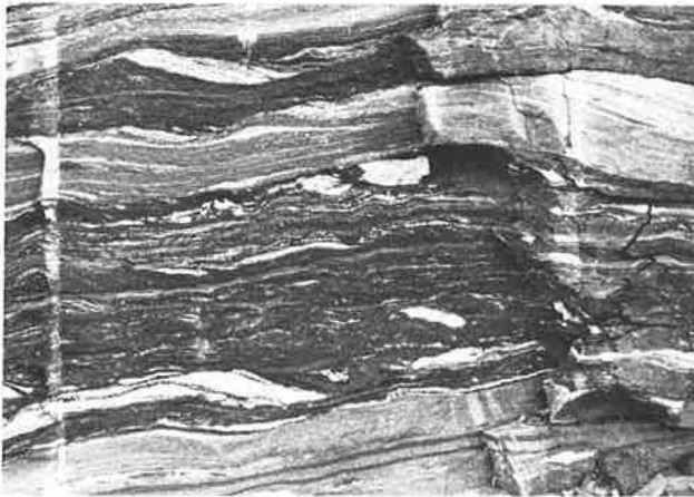
Figure 2. Banded gneiss freshly exposed in presplit highway cut: top to bottom 3 ft.
