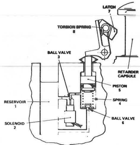
Figure 11. Prototype hold-down latches, Seinajoki Yard.
