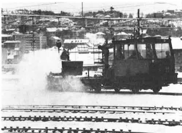
Figure 7. Snow-clearing machine at work, Trondheim Yard.
