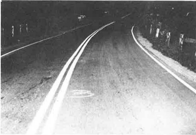
Figure 5. Condition of standard line (left) and commercial premixed paint with 2.5 lb of glass beads per gallon dropped on (right): initially in May (top) and after 9 months in February (bottom).
