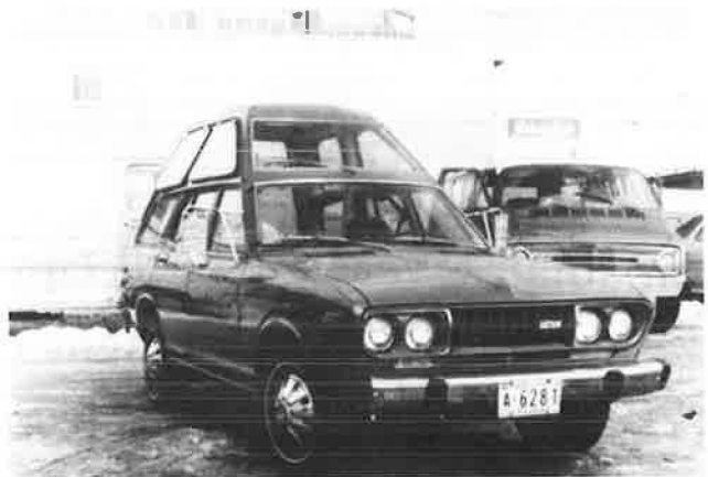
Figure 1. Datsun 710 subcompact station wagon modified by TDC for use by wheelchair passengers.
