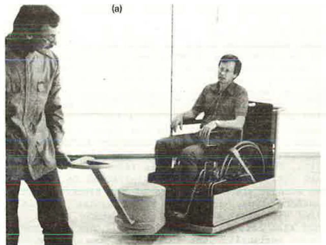
Figure 6. TDC modular transfer vehicle for use in terminals (a) for the wheelchair traveler and (b) for the ambulatory passenger, with second platform for luggage.
