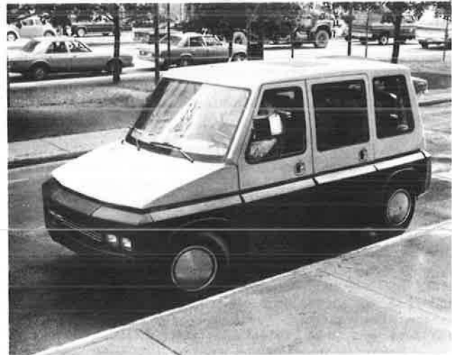
Figure 2. GSM taxi, which can carry one wheelchair passenger along with three ambulatory passengers.
