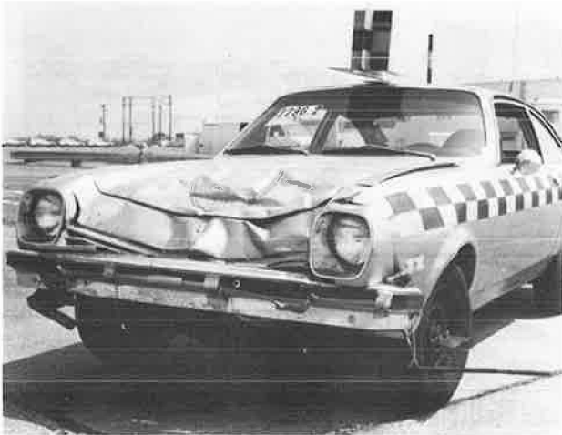
Figure 5. Test vehicle after test 2.
