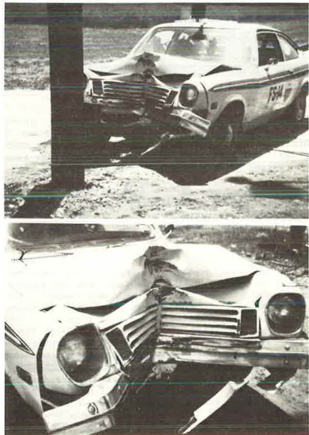
Figure 1. Unmodified pole crash test at 49 km/h.
