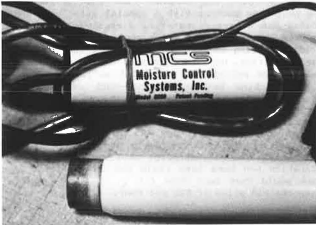
Figure 5. Moisture sensor timing and amplification module (top) and sensing module (bottom).
