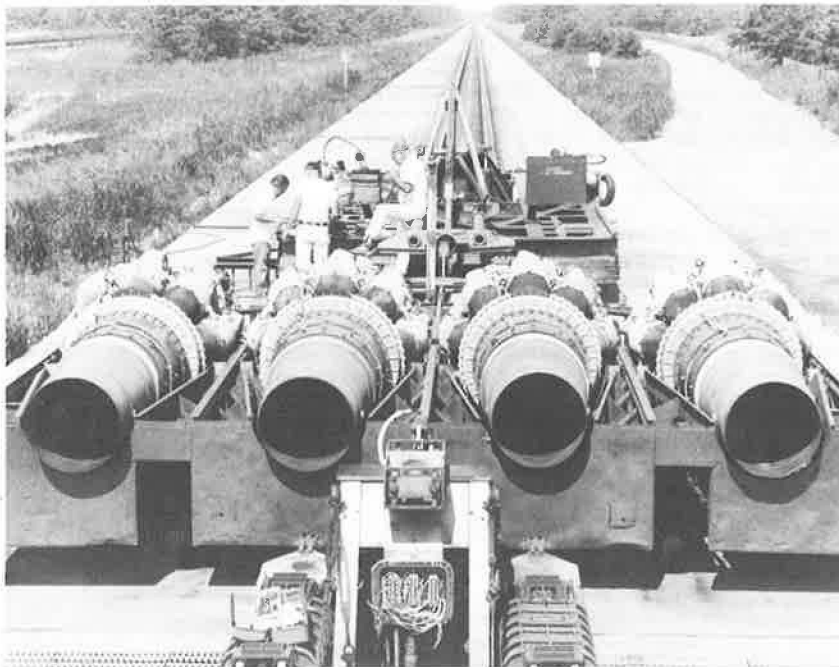
FIGURE 1 Jet-powered pusher car for providing preselected speed to test equipment.
