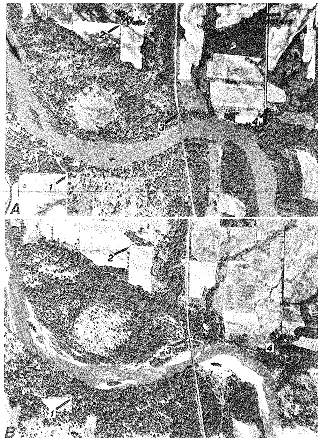
FIGURE 6 Examples of reference points on time-sequential aerial photographs. (A) Points, indicated by numbers, on 1969 photograph of Cedar River, Iowa. (B) Corresponding points on 1937 photograph. (U.S. Dept. of Agriculture photographs).
