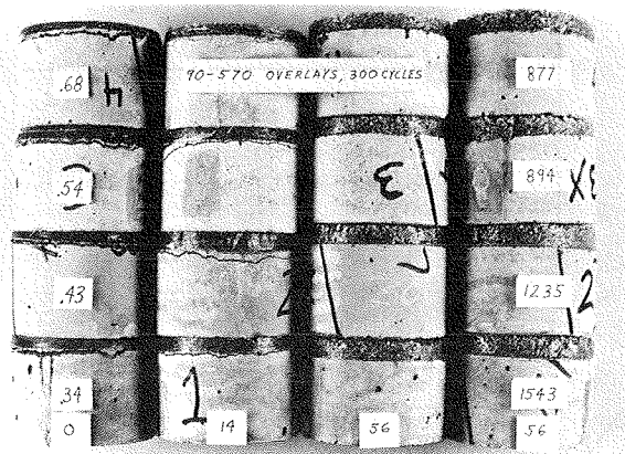
FIGURE 5 Condition of test specimens after 300 thermal cycles.
