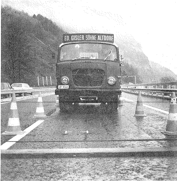
FIGURE 1 A two-axle vehicle before passing over a contact threshold (speed measurement) and over a 45 mm (1.8 in.) thick plank.
