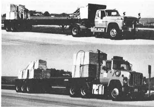
FIGURE 2 Trucks used: 18-kip SAL and 34-kip TAL (top), 42-kip TAL and 42-kip tridem-axle load (bottom).
