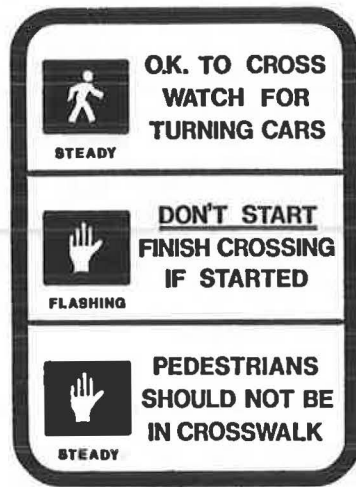
FIGURE 2 Devices tested to indicate the clearance interval: symbolic pedestrian signal explanation sign (left) and DONT START signal display (right).
