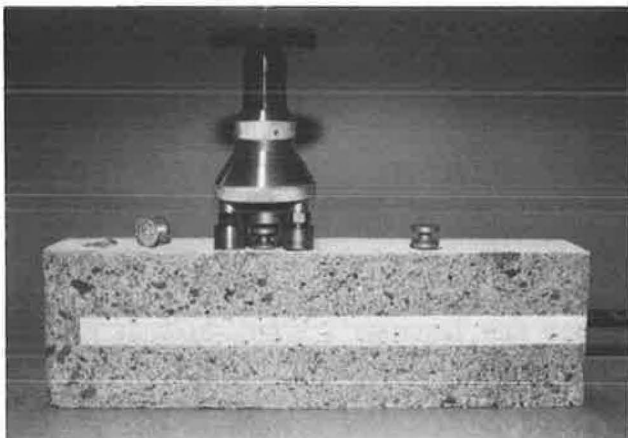
FIGURE 3 Adhesion tester and dollies on coated concrete.
