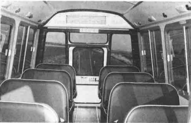
FIGURE 6 Emergency exit signage and instructions on a body-on-chassis small bus.
