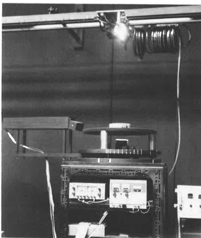
FIGURE 6 Photograph of equipment—the reflectance matrix photometer.
