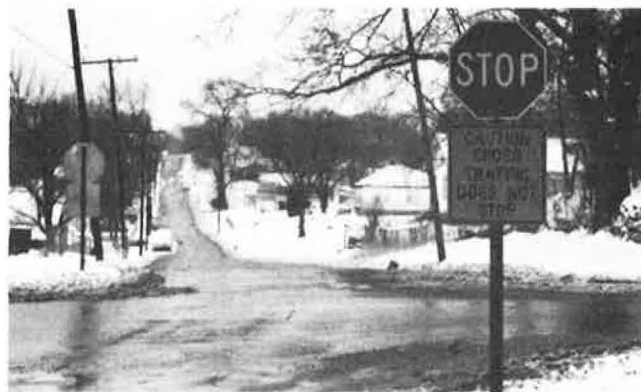
FIGURE 3 Supplementary sign after conversion (Kansas City, Missouri). Note supplementary sign on post on opposite corner.
