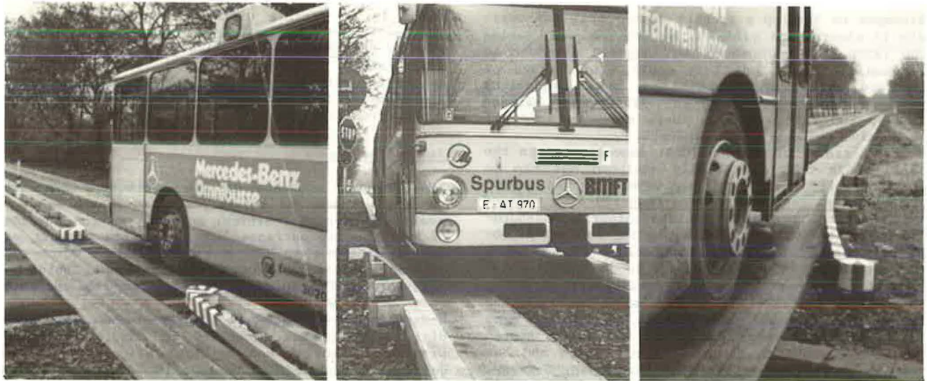
FIGURE 2 O-Bahn guideway entrance (1).
