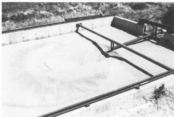
FIGURE 3 Model test stand for evaluating scour from sloping culverts.
