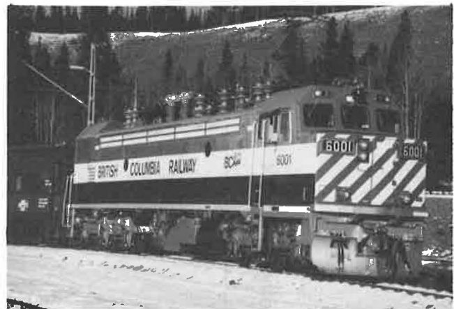
FIGURE 5 6,000-hp GF6C locomotive.
