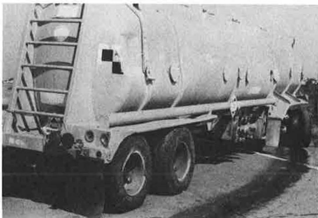
FIGURE 8 Tank truck weighing 80,000 lb after test.
