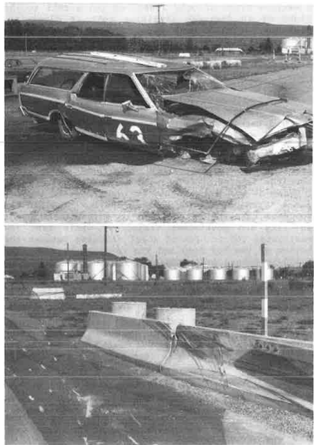
FIGURE 7 Test vehicle and barrier after Test 63.
