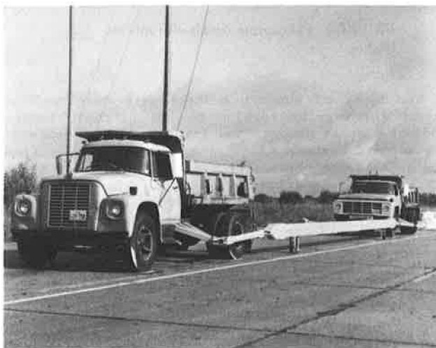
FIGURE 1 Truck-mounted portable maintenance barrier.
