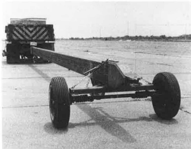
FIGURE 10 Barrier section on transport dolly.
