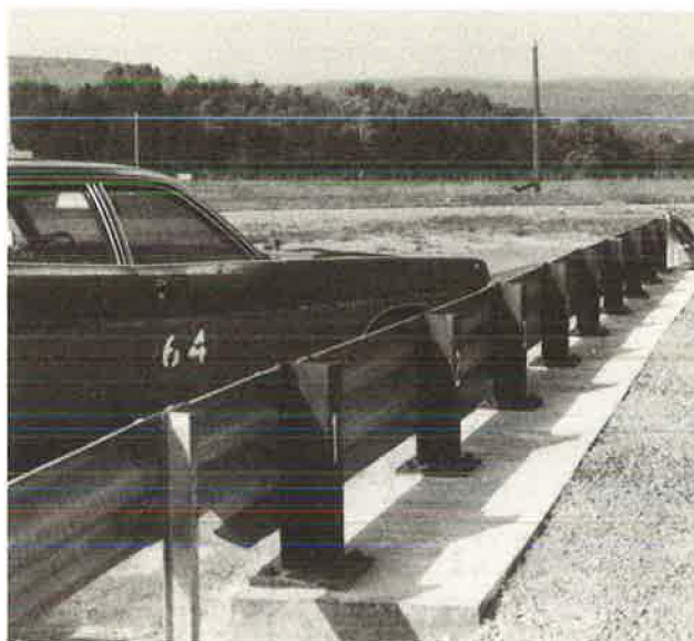
FIGURE 1 Thrie beam mounted on W6x25 post for Test 64.
