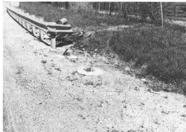
FIGURE 3 Proper performance of BCT end treatment.
