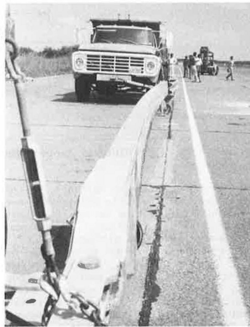
Figure 14 Accumulated damage to barrier section in Tests 1, 2, and 3.
