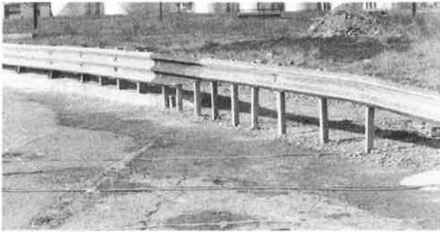
FIGURE 5 W-beam-to-thrie-beam transition evaluated in Test 68.
