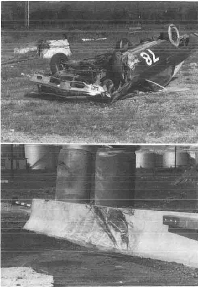
FIGURE 10 Test vehicle and barrier after Test 78.
