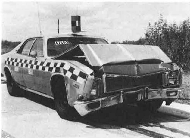
FIGURE 12 Frontal damage sustained by vehicle in Test 7.
