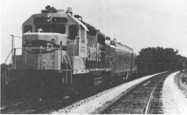
FIGURE 2 Santa Fe consist used for the long tangent test in Kansas.
