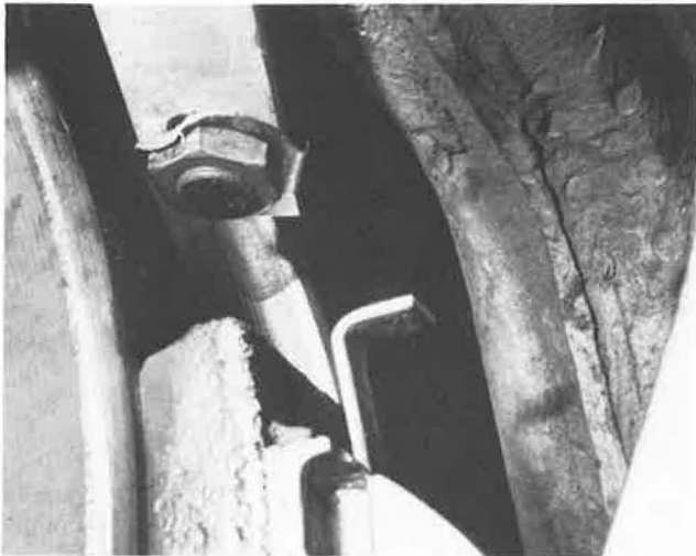
FIGURE 12 Spray nozzle, bracket, and grease spray pattern.
