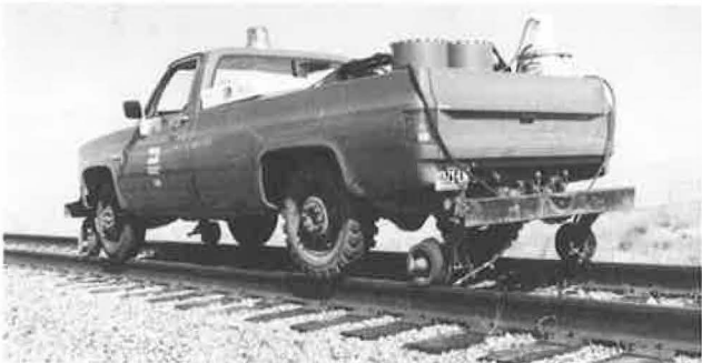
FIGURE 9 Lubricator system mounted in Hyrailer truckbed.
