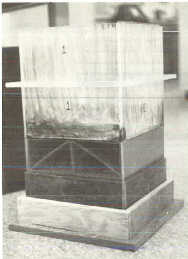
FIGURE 6 Deformation of carton form—test setup before placing of concrete.
