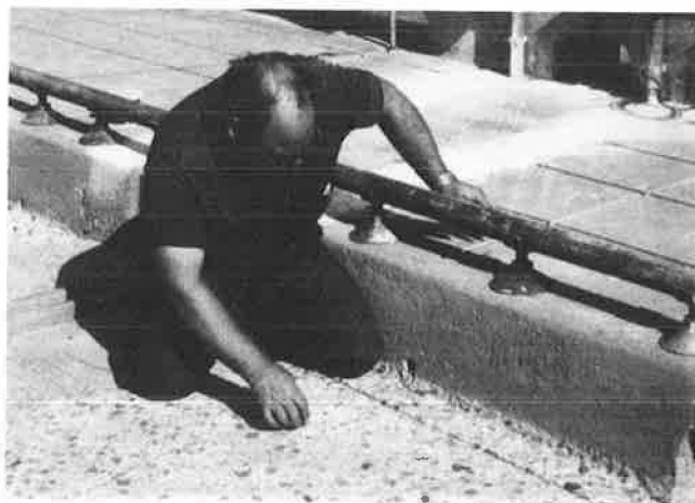
FIGURE 10 Passing platinum wire through curb.
