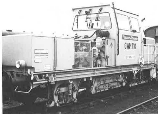
FIGURE 13 Plasser's shuffle grinder.
