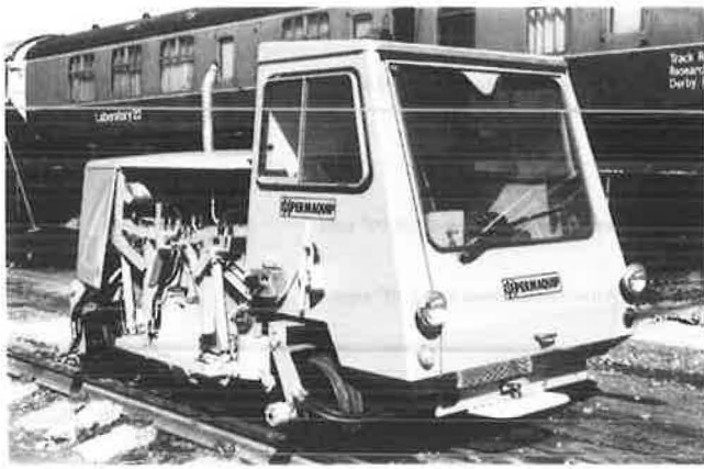
FIGURE 14 RASTIC's rail-bending machine.
