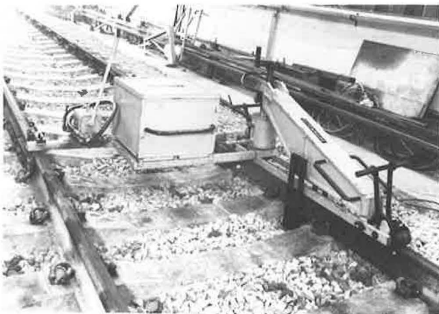
FIGURE 8 Three-point rail straightener.
