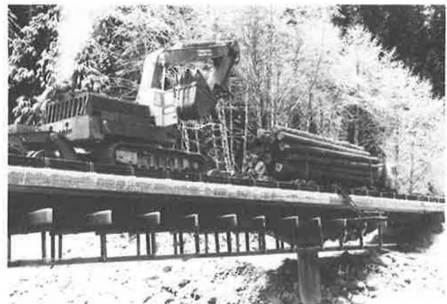
FIGURE 6 Photograph of two test vehicles applied simultaneously back-to-back during LP6.
