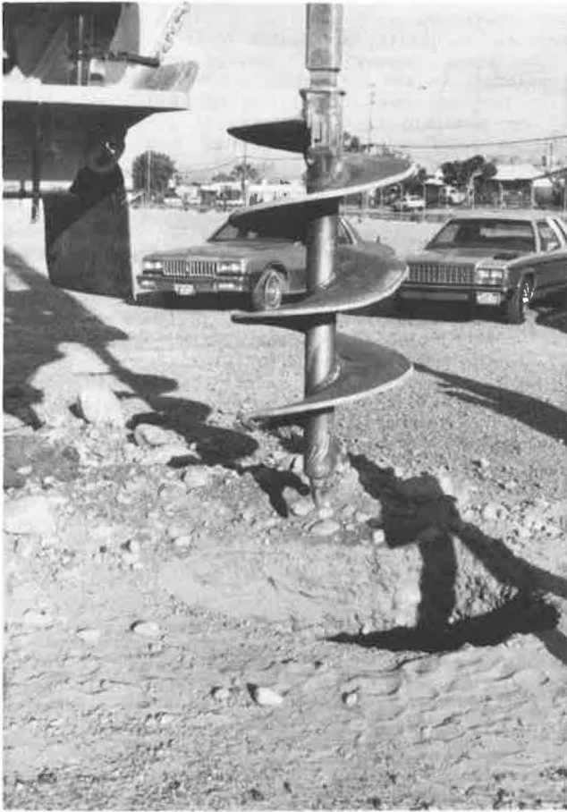
FIGURE 1 A 36-in. helical auger for large observation borings.
