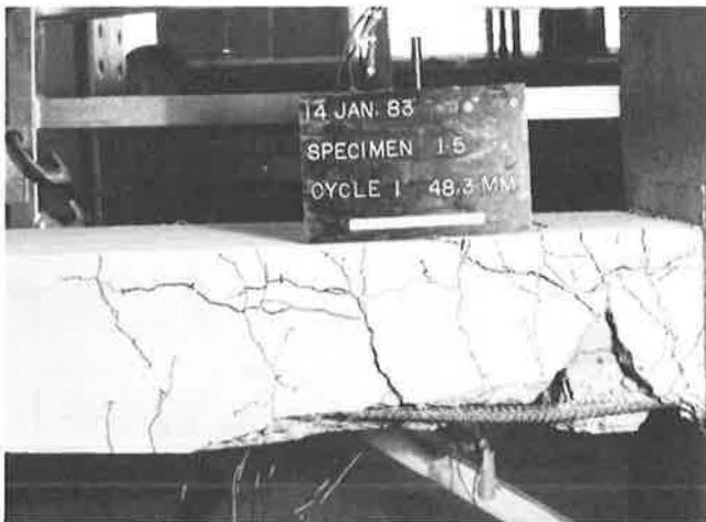
FIGURE 9 Final crack pattern for Specimen 1-5, 7δy/l.
