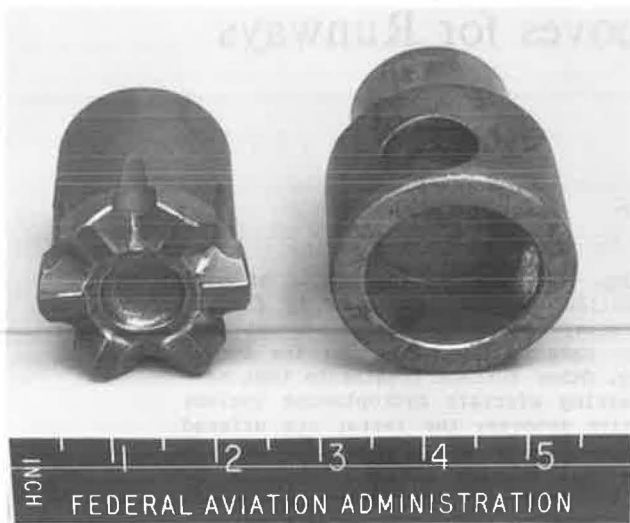
FIGURE 1 Original and modified cutting heads for installing reflex-percussive grooves.
