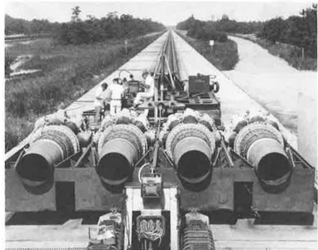
FIGURE 6 Jet-powered pusher car for providing preselected speeds to test equipment.
