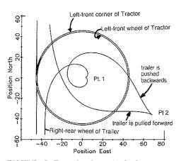
FIGURE 13 Example of a trailer backing up when attempting a continued short-radius turn.
