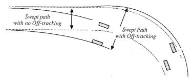
FIGURE 1 Example of the offtracking effect for a single-unit vehicle.
