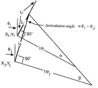
FIGURE 9 Computation of curvature of rear axle.
