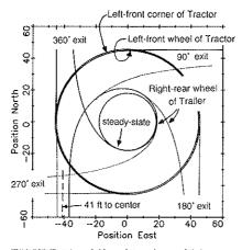
FIGURE 12 Offtracking for a 65-ft doubles combination vehicle in a 41-ftradius turn (45 ft to the outside front wheel).
