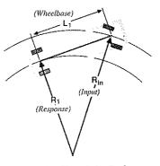
FIGURE 3 Use of the Pythagorean theorem to compute maximum (steady-state) offtracking in a constant-radius turn.
