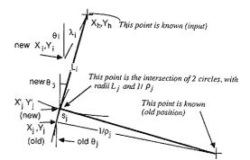
FIGURE 10 Calculation of new position of rear axle.
