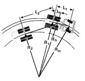
FIGURE 4 Use of the Pythagorean theorem to analyze maximum (steady-state) offtracking of a tractorsemitrailer in a constant-radius turn. is used consecutively to next calculate the radius of the path traced by the hitch
