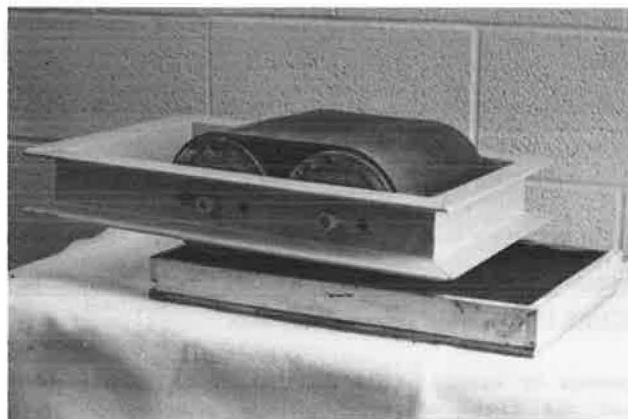
FIGURE 21 The developed new compactor (AMIR).
