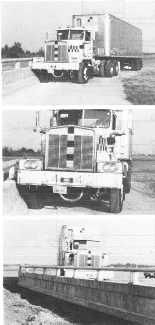
FIGURE 5 Comparison of 80,000-lb van-type truck and modified T5 bridge rail.
