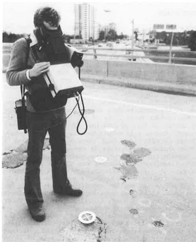
FIGURE 4 Infrared thermovision equipment being operated at ground level.
