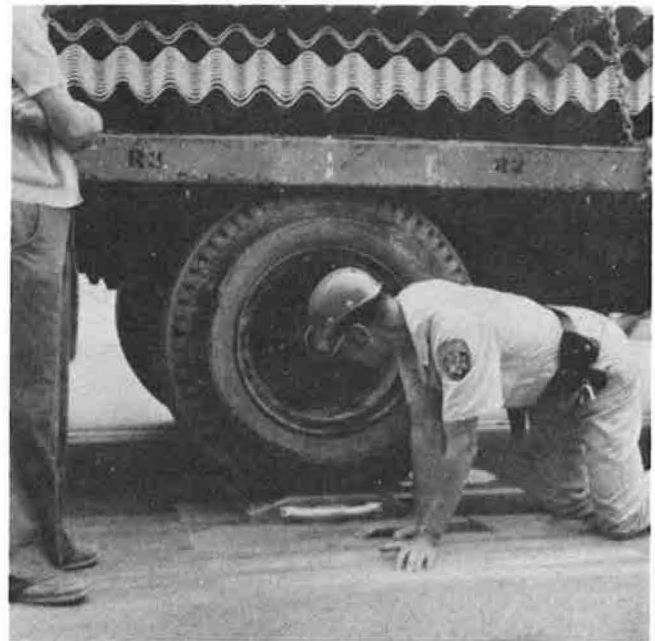
FIGURE 7 Stenner Creek—measuring wheel load.
