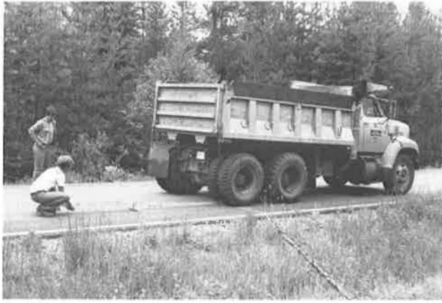
FIGURE 13 Benkelman beam deflection testing, Site D2-92-45.2.
