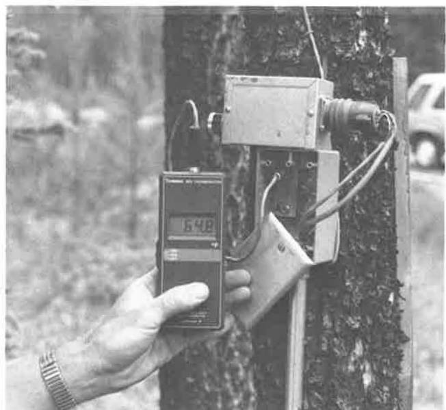
FIGURE 10 Electronic thermometer reading the 4-ft sensor, Site D2-92-45.2.
